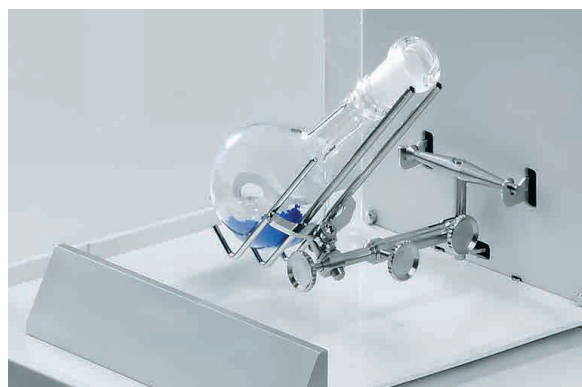
Figure 3: ErgoClip with flask on an XP56 analytical balance
