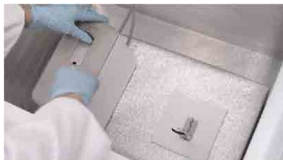
Figure 14: The external DP90 measurement cell in a freezer.
