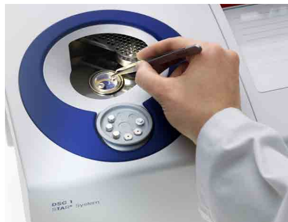
Figure 22: Manually placing a sample in the DSC furnace
