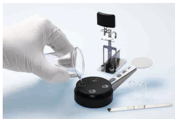
Figure 15: The DP sample preparation tool allows to fill the cups simultaneously with four samples.
