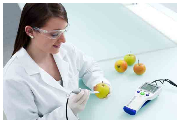
Figure 10: Use of a portable pH meter with puncture electrode to check pH value of apples
