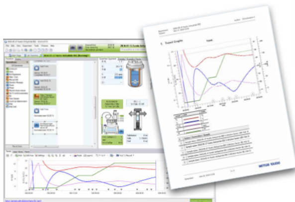
Simple recipe programming including sampling tasks in iControl software. Sampling events are annotated on the trend graph.
